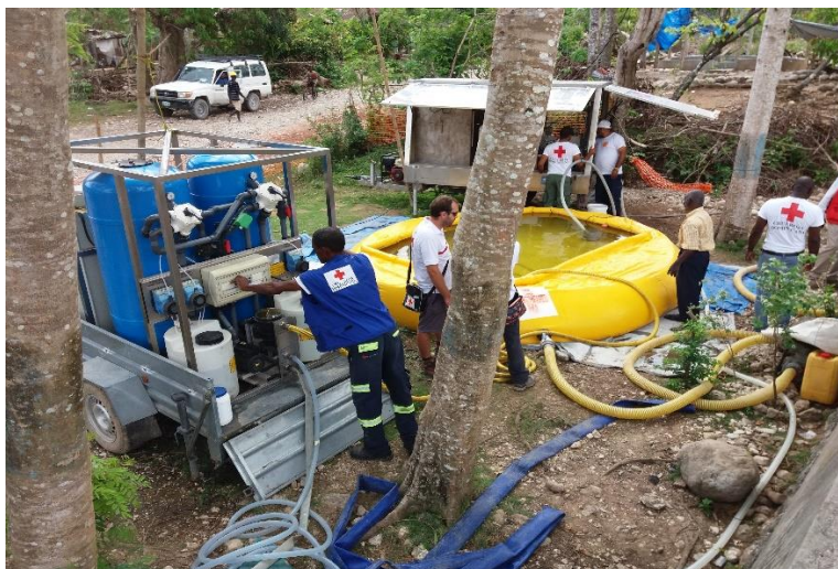
The Red Cross installed a mobile and temporary water treatment station in the field to facilitate the production and distribution of potable water to affected people. Source: IFRC
