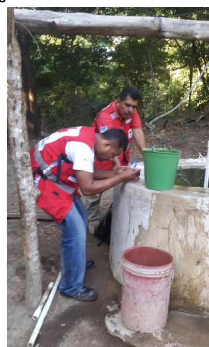
NRC personnel conduct turbidity and PH tests on the community of Ochomogo (Rivas departments)'s water supply. Source: NRC
