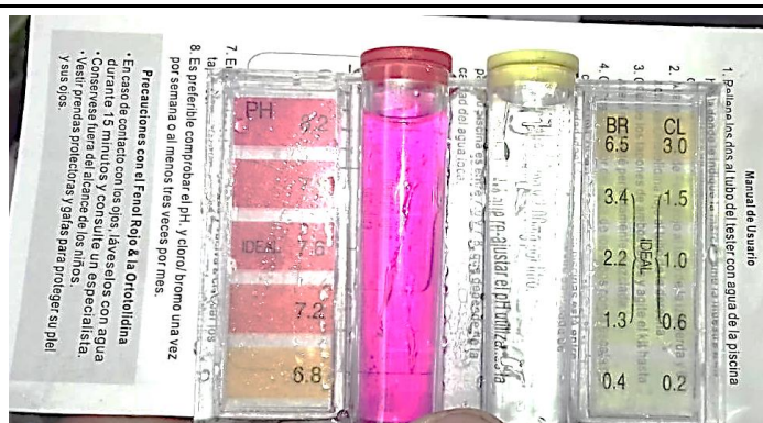
A pH test performed on the main source of water of the community of Amatal in Sonsonate.
