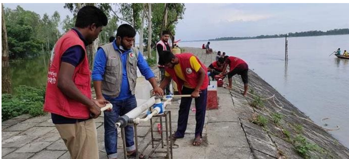
Red Crescent volunteers are preparing the water purification unit (Man-pack) on riverbank in Kurigram to provide safe drinking water to flood affected people. (Photo: BDRCS)
