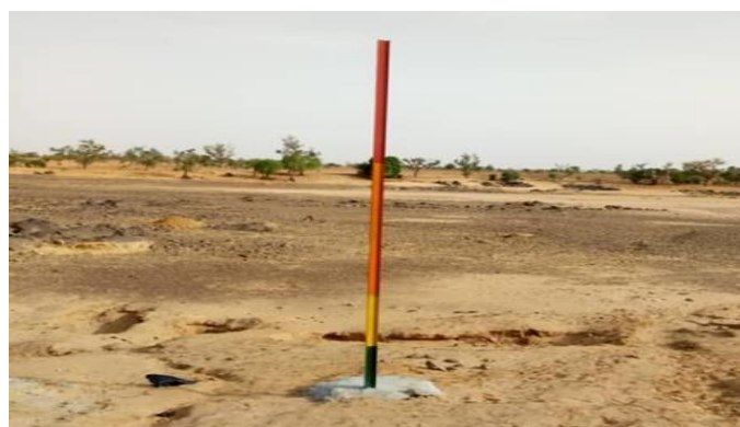
Figure N°2: Colorful scale serving as a beacon of alert for communities in the Sirba Basin. @Ministry of Water resources, Niger
