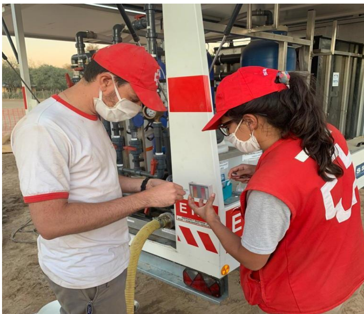
Testing water pH for production of safe water, ERU. Source: Argentine Red Cross.
