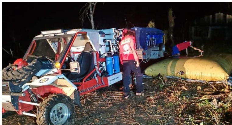
Water treatment units including our desalination unit set-up for safe water distribution in Bato, Catanduanes. PRC could treat brackish water and make it potable for the people affected (Photo: PRC)
