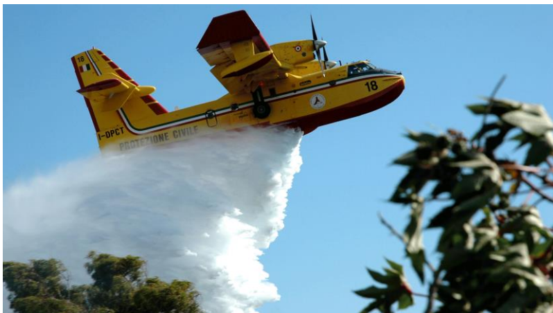
Photo 2. Firefighting aircraft (Canadair CL415) dropping water on wildfires in Abbasanta. Source: Sardinia Regional Government
