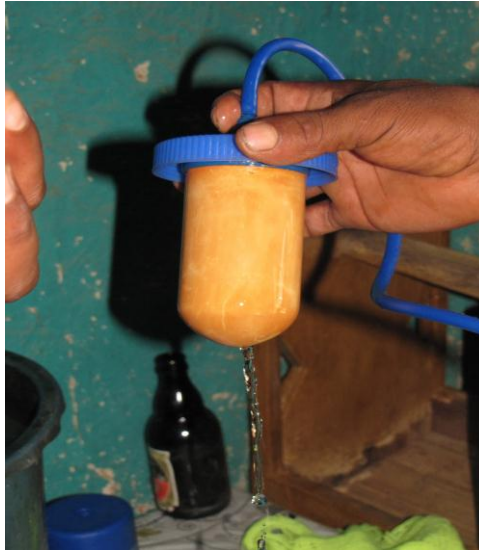
Tulip water purification filter and demonstration of how the tulip filter is used in the Dawa community/IFRC
