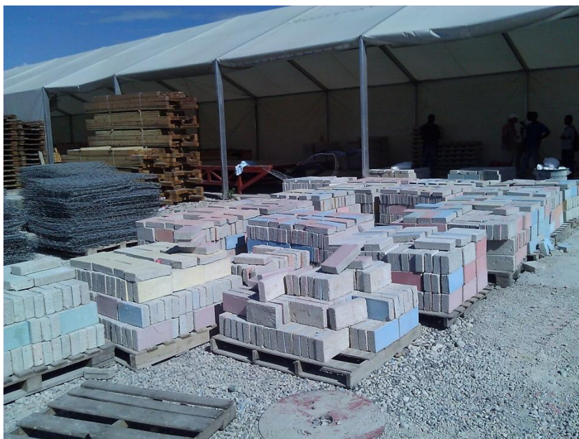
IFRC paving slabs made from reprocessed rubble
