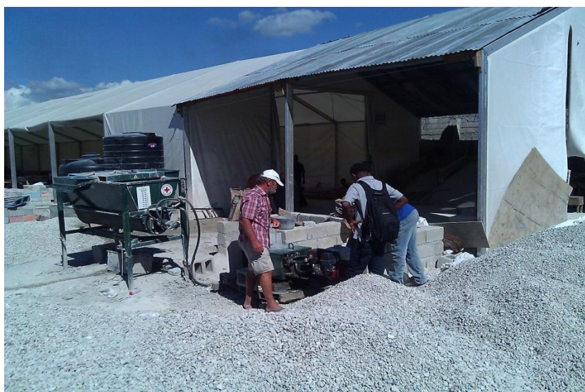
Aggregate produced from earthquake rubble
