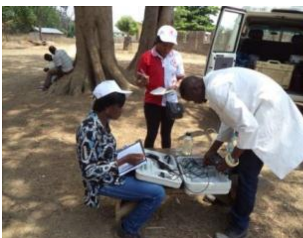
Collection of water sample and physical parameter analysis at one of the Odogwu community water points (open well)
