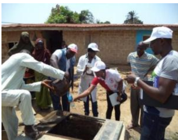
Collection of water sample and physical parameter analysis at one of the Odogwu community water points (open well)
